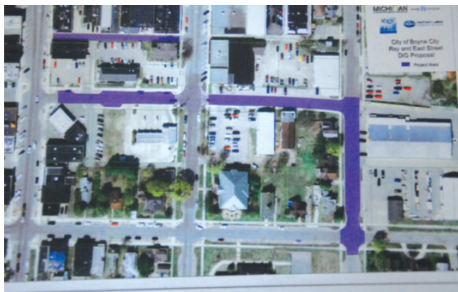
The roads highlighted in purple are the streets that the city has targeted for reconstruction.
